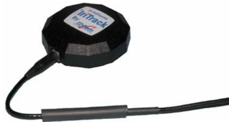
Iridium Module Leads connected with Heat Shrink Tube in place
