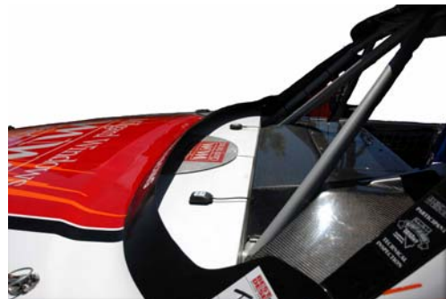
Optimal Antenna Location Is A "No Crush Zone"
